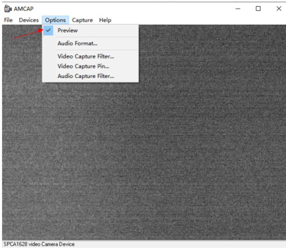
**When connect successfully, you will see the screen of the night vision device turns white, and you will see the contents on your computer, please rotate the objective lens of the night vision device to focus on to see the objects clearly.**
